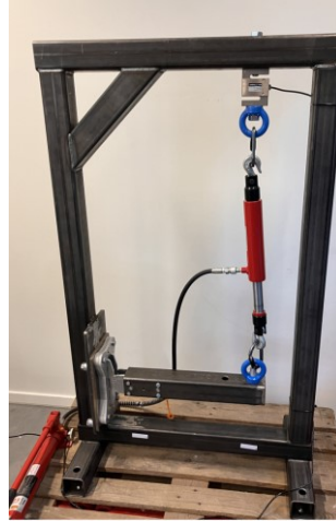
Figure 1 - Test rig with means to apply forces
